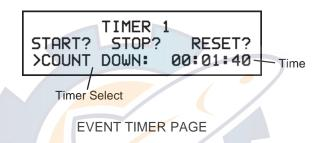
The GPS 100 features two timers available on separate pages. Each can be used as either an elapsed timer or count down timer. These timers can be useful for measuring the elapsed time since a certain event, or they can tell you when a specified amount of time has expired.
